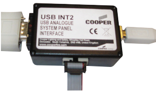
TTL to USB - Wireless survey tool connection
