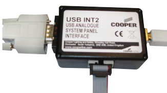
TTL to RS232 - Wireless survey tool connection (serial link)
