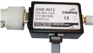
RS232 to USB - Wireless panel to PC (site installer)
