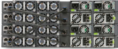
Rear View (demonstrating Stackable Chassis cabling)
