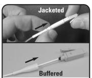
Simplex cable only Slide the boot up into place onto the crimp sleeve (jacketed fiber) or connector housing barrel (buffered fiber). For duplex jacketed cable, do not slide boots up until after polishing is complete.
