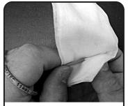
Using a dry, lint-free wipe; Remove any remnants of the protective coating on the fiber after stripping the buffer.
