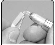
Hold the flat surface of the scribe 11 tool flat against the ferrule tip with the beveled edge facing up. Carefully score the fiber close to the intersection of the ferrule tip and fiber. Score on one side only. Clean the adhesive off blade.
