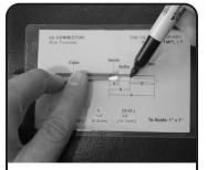
Using the marker pen and the template card provided, measure and mark the buffer strip length as shown on the template.
