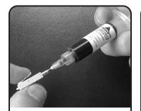
Remove dust cap from the connector and insert the adhesive syringe tip into connector housing until it seats firmly inside. Inject the LightSpeed adhesive until a small dot of the adhesive appears at the ferrule tip. Also inject a small amount of adhesive into the back end of the connector. This ensures bonding of the buffer to the connector, strengthening the termination. Be careful not to overfill to prevent a backflow of adhesive.
