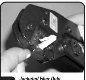
Slide the crimp sleeve up over the kevlar so that it is seated against the shoulder of the connector housing, being sure the sleeve does not move prior to being crimped. Position the crimp tool over the crimp sleeve using the 0.12 in. opening in the crimp die. Crimp the sleeve by closing the crimp tool completely and releasing. Crimp only once.
