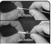
Insert the fiber into the connector until the buffer bottoms out inside the housing. Allow at least 30 seconds cure time before proceeding. Tip: Rotate the connector during insertion to assist in guiding the fiber into the ferrule. For jacketed fiber, allow the kevlar to fan out around the connector barrel.
