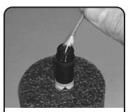
Insert primer bottle into the stand. Dip the entire exposed fiber into the LightSpeed® primer and place in a protected area.
