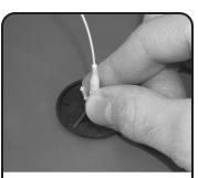
Gently grip the connector and apply medium pressure and polish in a 50-75mm [2-3 in.] "figure 8" pattern for 25 to 30 revolutions.
