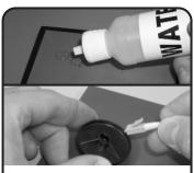
Add a minimum of 3 or 4 drops of distilled/deionized water on the polishing film and carefully insert the connector ferrule into the LC compatible polishing puck (provided with the FTERM-LC) and gently place on pad. Avoid bumping ferule tip on puck or crushing exposed fiber onto pad.
