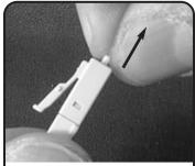
Remove the excess fiber with a straight, non-twisting pull and deposit in a safe place (i.e. onto a piece of tape or in the debris container).
