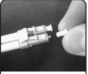
Replace dust caps onto the connector ferrules while connectors are not in use.
