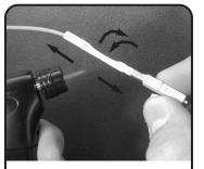
Jacketed Fiber Only Using the small propane torch from the FTERM-LC or equivalent, carefully heat up the shrink tubing on all sides to provide proper strain relief.
