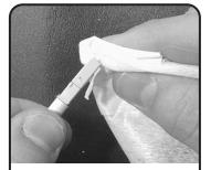
Prior to viewing endface of connector with microscope clean with a dry lint-free wipe.
