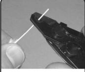
Using the buffer strippers, strip off the buffer in at least two pieces.
