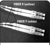
Note: To ensure proper transmitter-to-receiver patching, be certain to assemble each end of a duplex assembly with the opposing orientation as shown. To help identify proper orientation it is helpful to place the same color shrink tubing on opposite end of the same fiber strand. If correctly assembled the final duplex assembly will have opposite color-coded strands on the A side as well as the B side.
