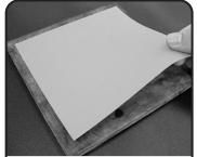
Place the polishing pad onto a flat surface with the rubber side facing up. Place the #2 film onto the polishing pad with the glossy side of film down. Note: Prior to polishing, clean pad surface with alcohol soaked wipe to provide for a smooth polishing surface. This will also allow the polishing paper to stick in place. (Ensure no air is trapped between pad and film). Also clean polishing puck.
