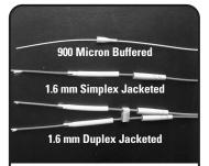
Slide the strain relief boot (and crimp sleeve for jacketed fiber) over the fiber in the proper orientation as shown. For duplex LC connectors, orient the A/B clip with the letters facing the strain relief boots as shown, also see step 29 for proper polarity.
