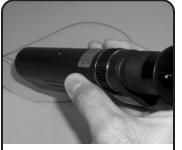
Using the microscope fitted with the LC compatible insert\*, inspect the polished surface for scratches, voids or chips. If polish is acceptable, place dust cap on connector.
